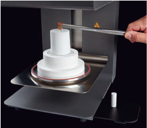
FIG 7: After the firing, VITA AMBRIA was pressed with the appropriate PLUNGER.
