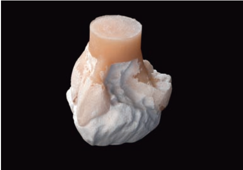
FIG 8: The investment material VITA AMBRIA INVEST generally ensures a completely minimal reaction layer.
